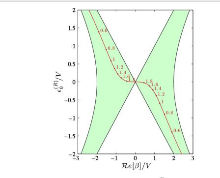
**Figure 4.** Band structure (green shadowed array) of the model equation (15) versus  $\epsilon_0^{(R)}$ . The red line indicates the trajectory of the defect eigenmode as  $\epsilon_0^{(R)}$  increases. The red dots and the associated numbers are indicative values of the critical  $|\epsilon_0^{(I)}|$  (for the specific  $\epsilon_0^{(R)}$ ) above which a defect mode is created.
